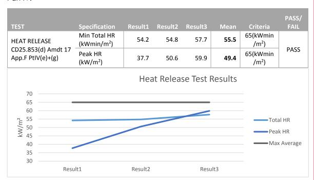
All three test pieces passed the Heat Release testing.
