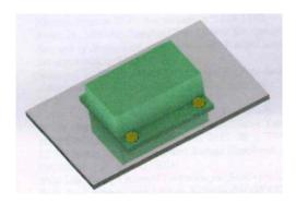
Tests were carried out on SATTO SA30-30, SATTO SA30-40 and EA934 (as a strength and cure comparison) in order to determine the shear strengths of the repaired joints after a 2 hour curing period, 7-day curing period and 28day curing period.
